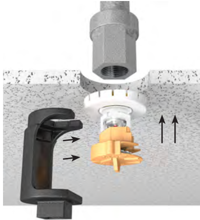
Figure 3: Recessed Installation (with Recessed Socket Wrench)
