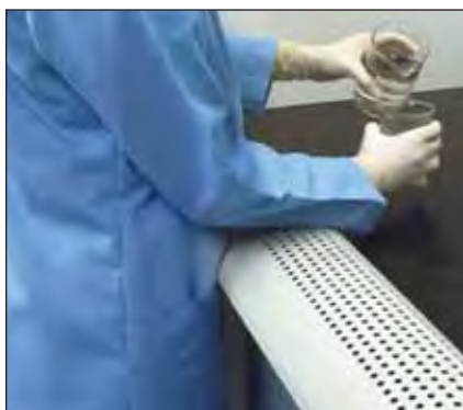
When the operator blocks the front of the air foil, air enters from under the air foil so "dead-air" zones are minimized and containment maintained.
