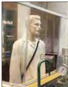
As part of ASHRAE 110-95, a tracer gas is released at an established rate and at various positions within the hood. The gas is monitored in the breathing zone of a mannequin placed at various positions in front of the hood. Based on the release rate of the tracer gas and the average exposure in the breathing zone, a performance rating is determined. An "As Manufactured" (AM) rating of 0.05 part per million (ppm) or less is considered effective containment.
