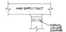
5 DETAIL SCALE: 1/4" = 1'-0" HARD DUCT BRANCH
