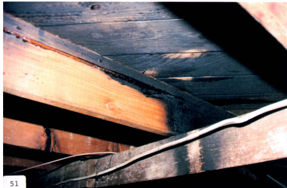
Figure 8 Floor burn-through in USFA test initiated by pouring gasoline on floor; limited ventilation (Test #6)
