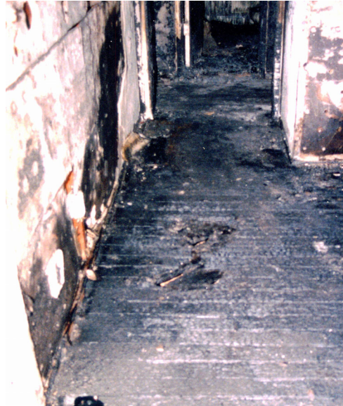
Figure 3 Floor burn-through in another Santa Ana Fire Dept. fire test; no liquids were used (Courtesy James C. Albers)
