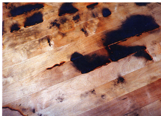
Figure 6 Char pattern from an 0.6 L gasoline pour onto a wood floor consisting of 25 mm maple floor boards, atop two layers of 13 mm plywood (Courtesy Fred Fisher)
