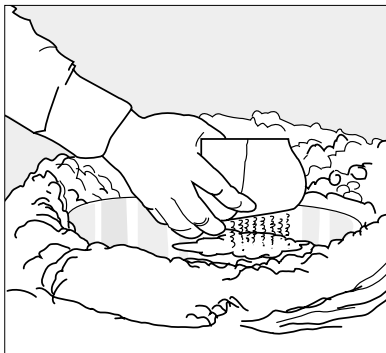
Sift gauging plaster into water
