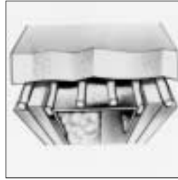
53 STC Sealed beneath and on edge of runner track. Base layer not relieved. Face layer relieved and sealed.
