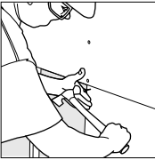
Nailing technique for single-layer application
