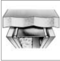
53 STC Both base layers sealed. No relief on face layers.
