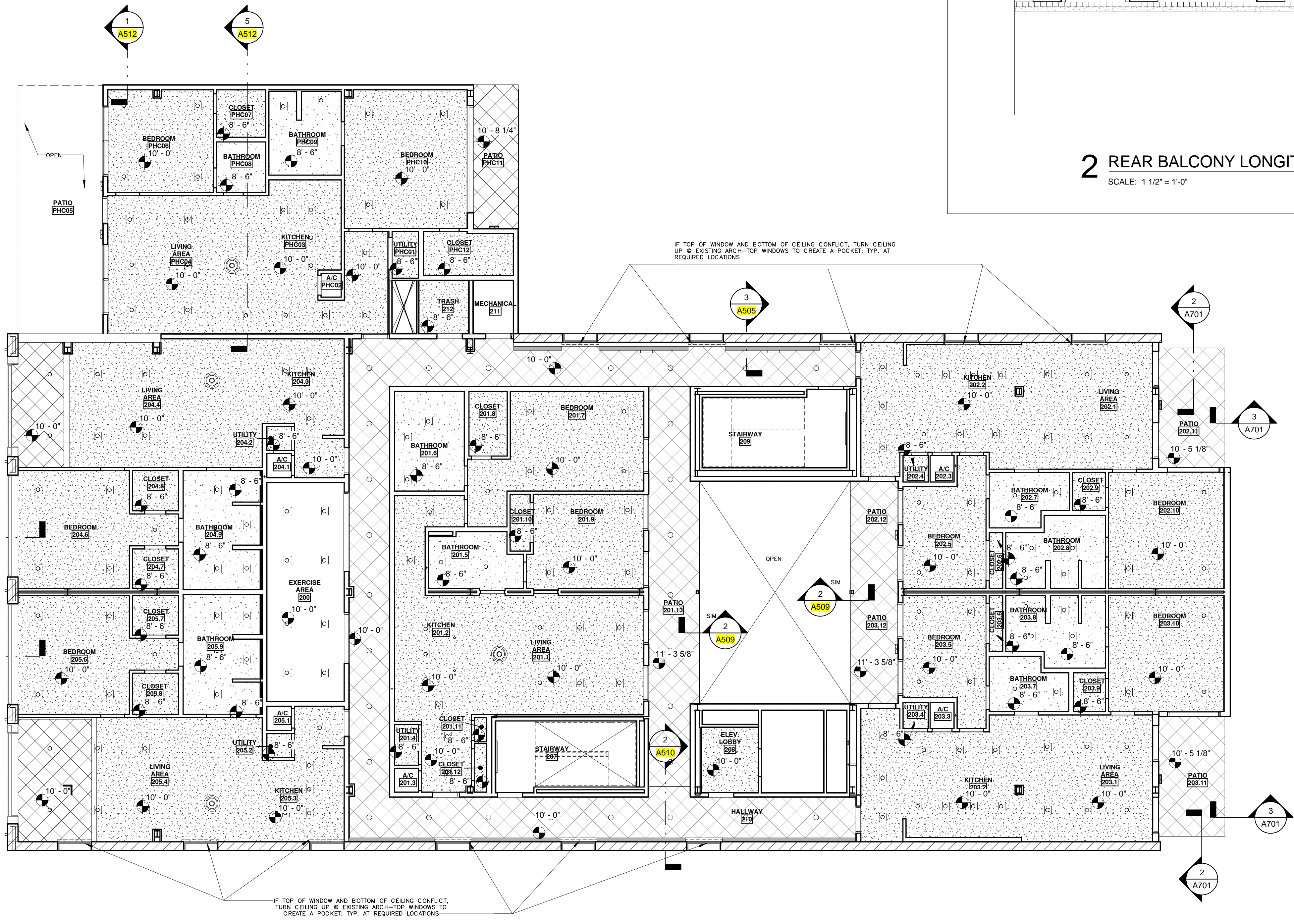
1 SECOND FLOOR REFLECTED CEILING PLAN SCALE: 1/8" = 1'-0"
