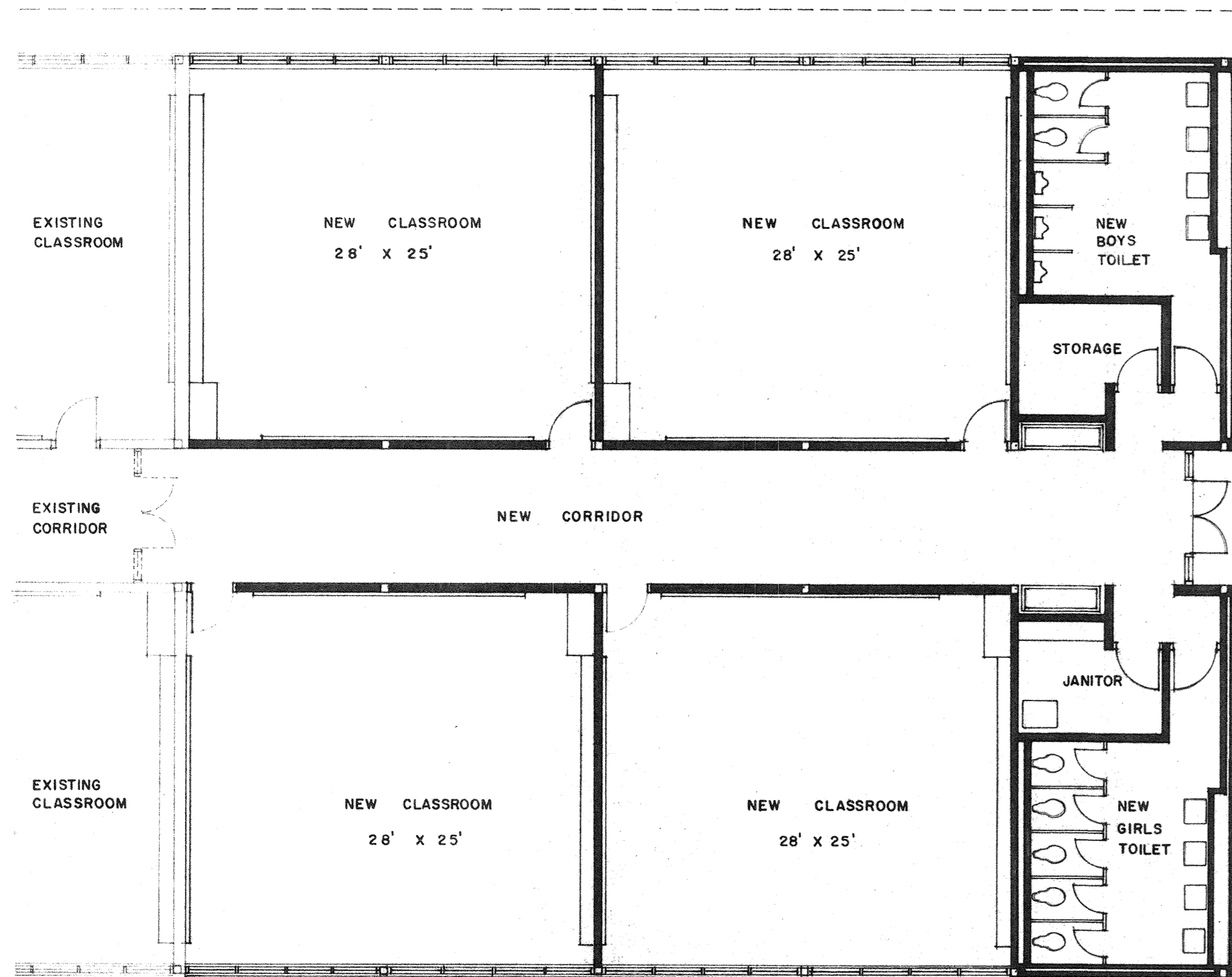
FLOOR PLAN - NEW CLASSROOM ADDITION - 4340 SQ. FT. SCALE: 1/8" = 1'-0"
