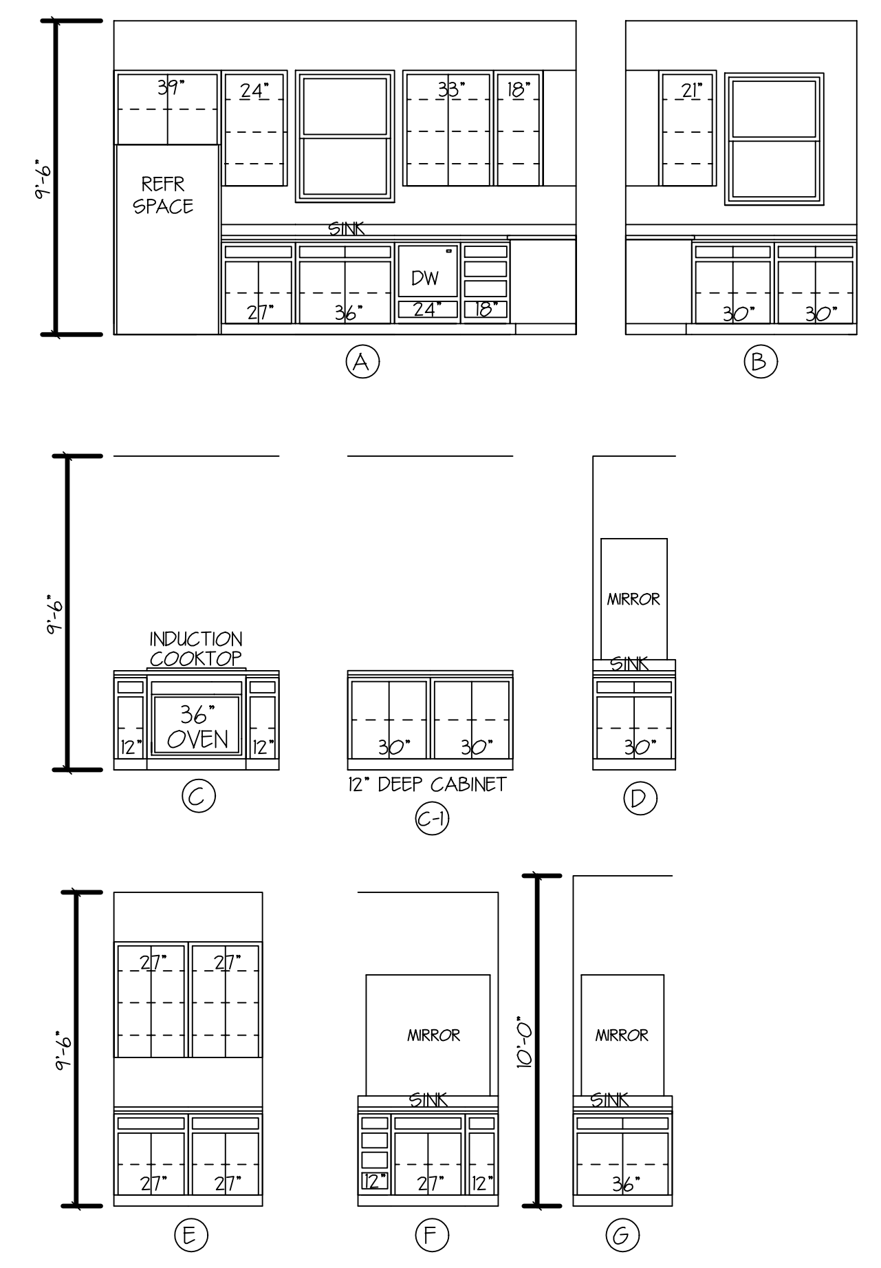
CABINET ELEVATIONS SCALE 1/4"=1'-0"
