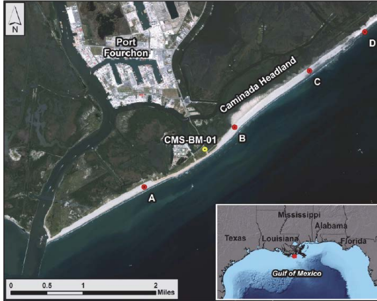
Figure 4-7: Station locations for sediment borings and anchor monuments for documenting subsurface sediment characteristics and monitoring elevation changes in response to beach restoration along Caminada Headland [23].
