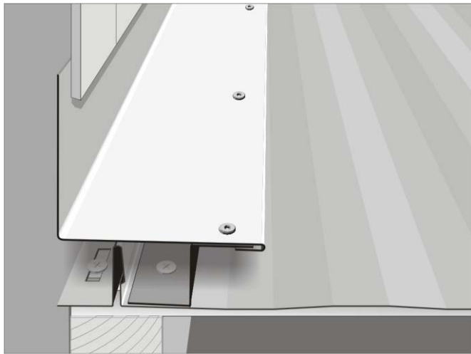
Fig. 17 Standard Sidewall attaches to z-flashing with rivets and is covered on the wall side by siding.
