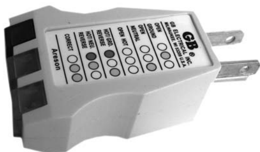
Figure 3-16 Plug-in outlet analyzer
