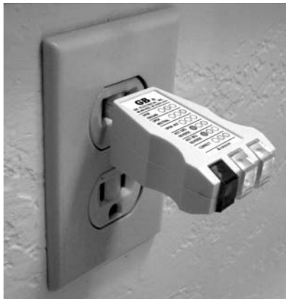
Figure 13-14 Using 120-volt outlet tester
