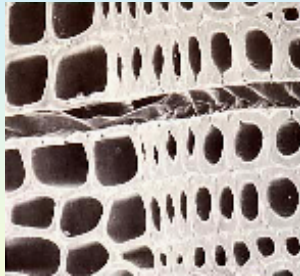
Normal regular and ray cells. Spring growth at left, summer at right.
