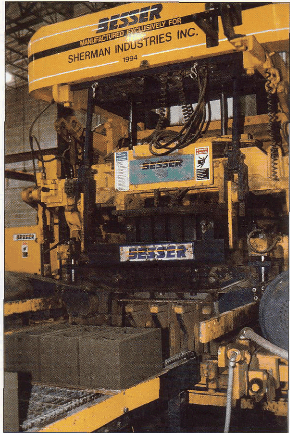
MANUFACTURING CONCRETE MASONRY Low-slump concrete is molded to the desired shape in hydraulic concrete products machines.
