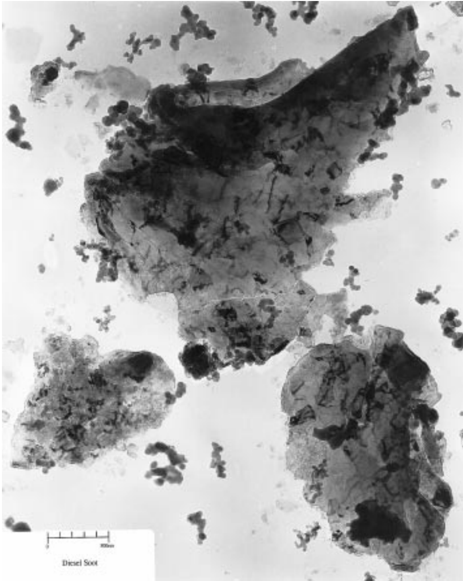
FIG. A1.8 Diesel Soot, Scale = 500 nm
