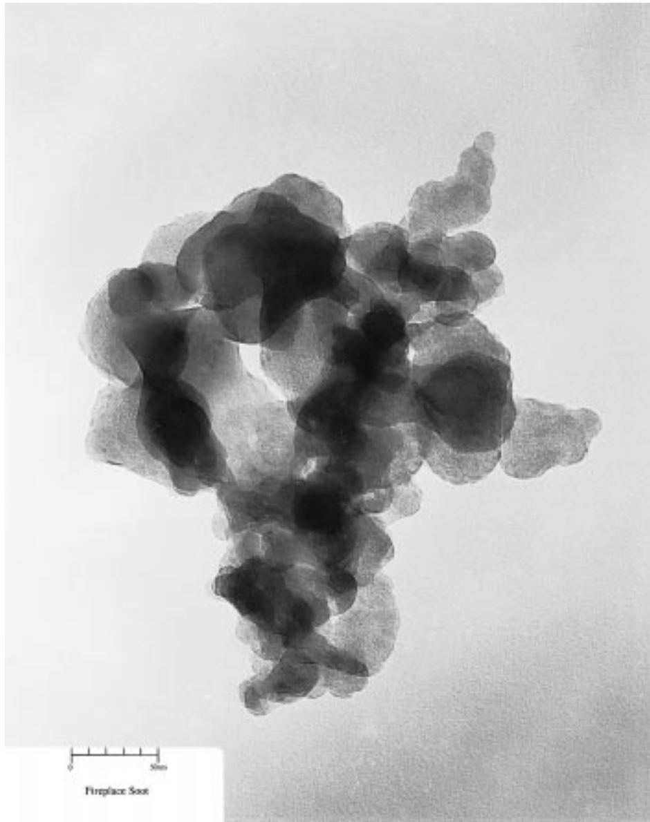
FIG. A1.5 Fireplace Soot, Scale = 50 nm
