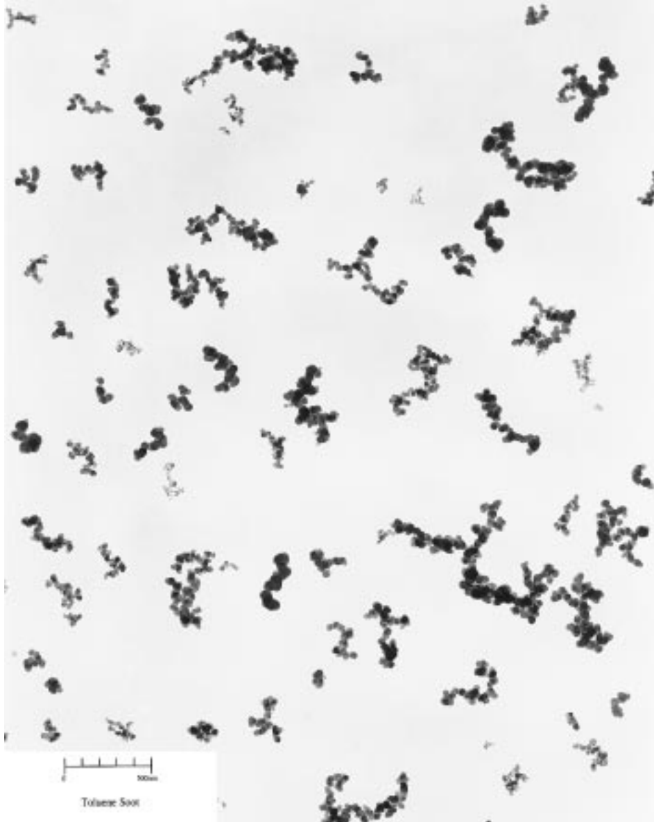
FIG. A1.4 Soot Produced in a Laboratory, Scale = 500 nm
