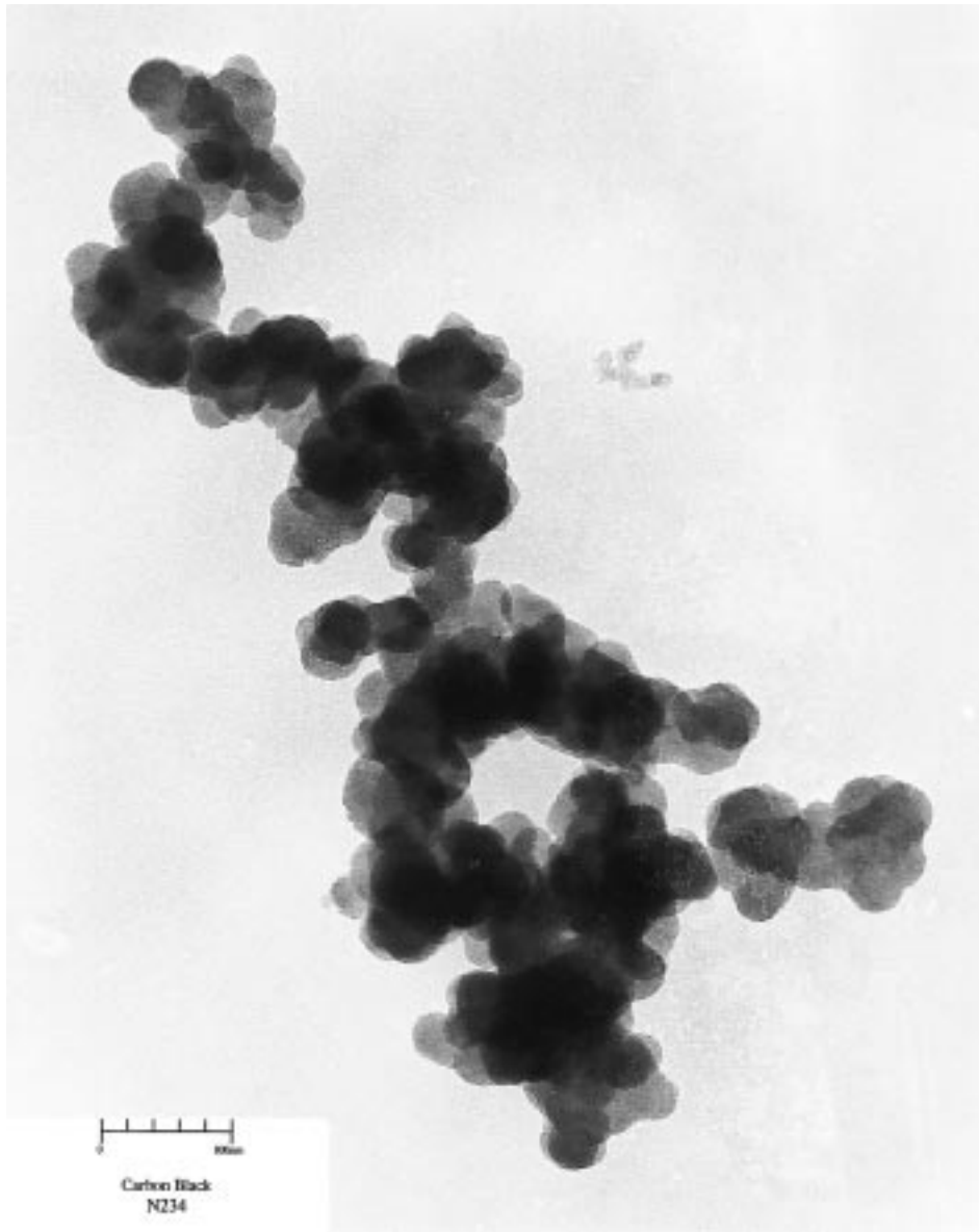
FIG. A1.10 N234 Carbon Black, Scale = 50 nm
