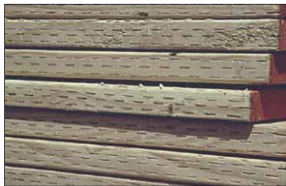
Incising is an aid in securing deeper and more uniform penetration of preservatives in western softwood species such as Douglas-fir, Hem-Fir and Spruce-Pine-Fir.
