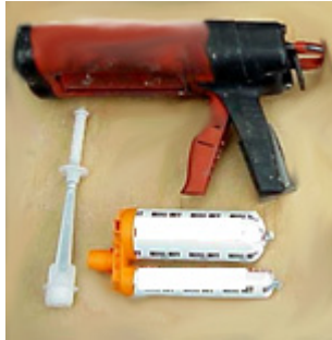
Fig. 4.1: Adhesive anchor system consisting of foil cartridge, mixing nozzle, dispensing tool, brush and hand pump (the MPII is not shown) (Courtesy of IWB, University of Stuttgart)
