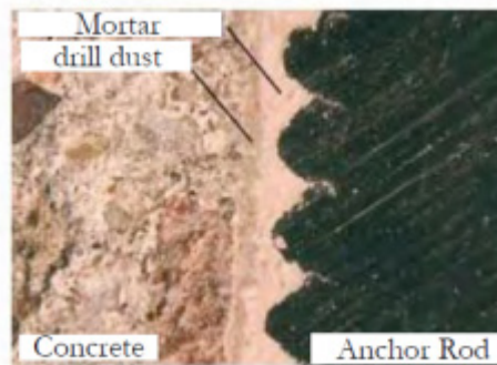
Fig. 4.2: Cut sections of installed adhesive anchors. The image on the right has a visible layer of drill dust that interferes with the bond between the epoxy mortar and the concrete. (Courtesy of IWB, University of Stuttgart)
