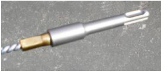
Fig. 4.8: SDS chuck, with brush attachment (brush top extends beyond left side of photograph), designed to fit into a drill
