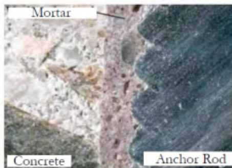
Fig. 4.2: Cut sections of installed adhesive anchors. The image on the right has a visible layer of drill dust that interferes with the bond between the epoxy mortar and the concrete. (Courtesy of IWB, University of Stuttgart)
