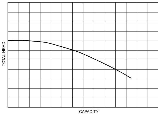
Fig. 12 Typical Pump Curve
