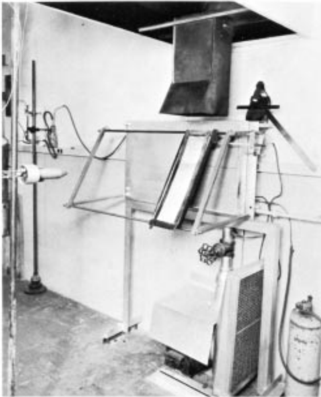
FIG. 1 Radiant Panel Flame Spread Test Equipment
