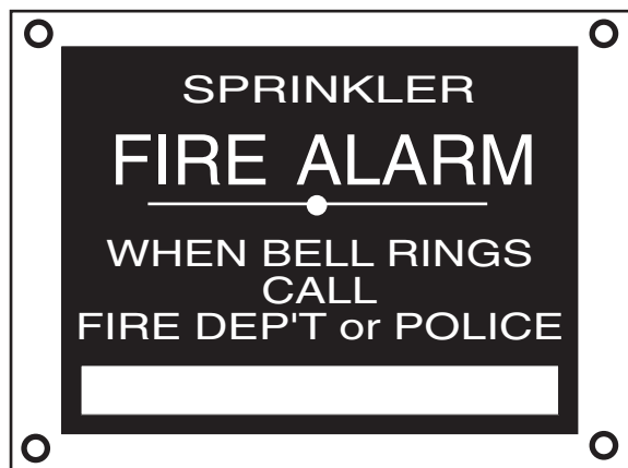
FIGURE A.8.17.1 Identification Sign.
