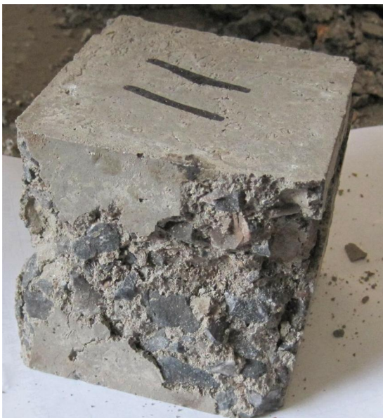
FIG. 7 PET concrete's cross section after test.
