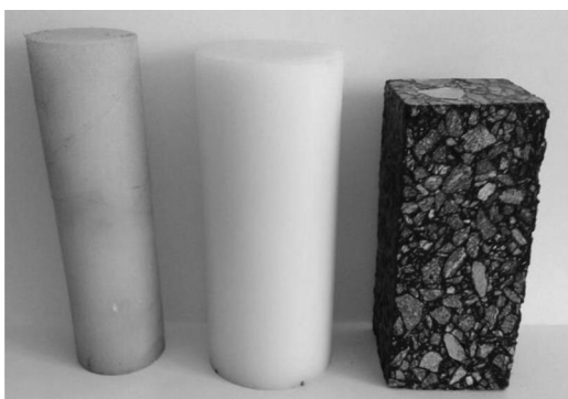
FIG. 1 Specimens made from polyethylene, polycaprolactam, and asphalt mixture (from left to right).
