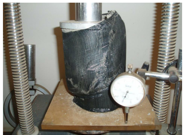
FIG. 12 The rupture of PP woven geotextile upon ultimate compressive strength.
