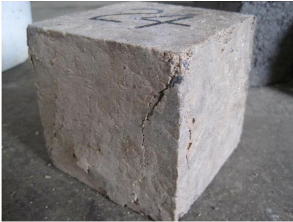
FIG. 6 Specimen after compressive strength test.
