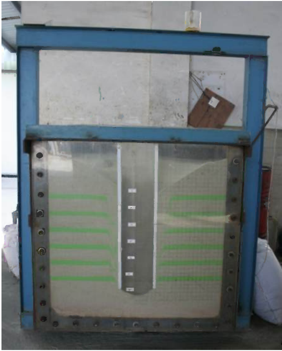
FIG. 2 Test box with the caisson.
