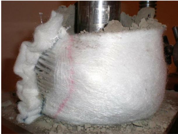
FIG. 13 The rupture of PET non-woven geotextile upon ultimate compressive strength.
