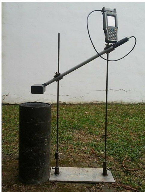
FIG. 3 Test equipment of manhole identification using RFID technology.
