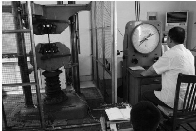
FIG. 1 Mechanical testing of HRBF400.
