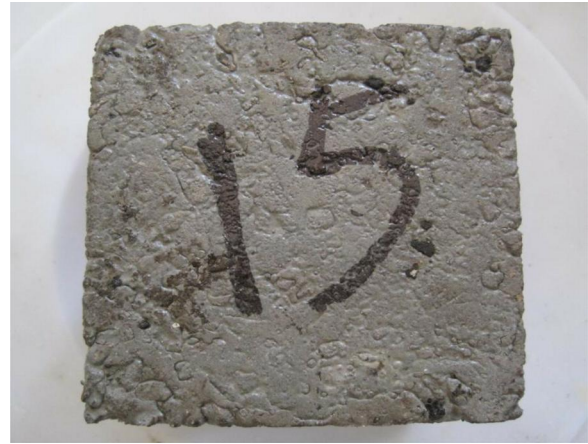
FIG. 4 PET concrete cube.
