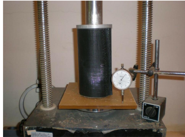
FIG. 7 Unconfined compressive strength test for hardened RS-CLSM sample reinforced with PP woven geotextile.
