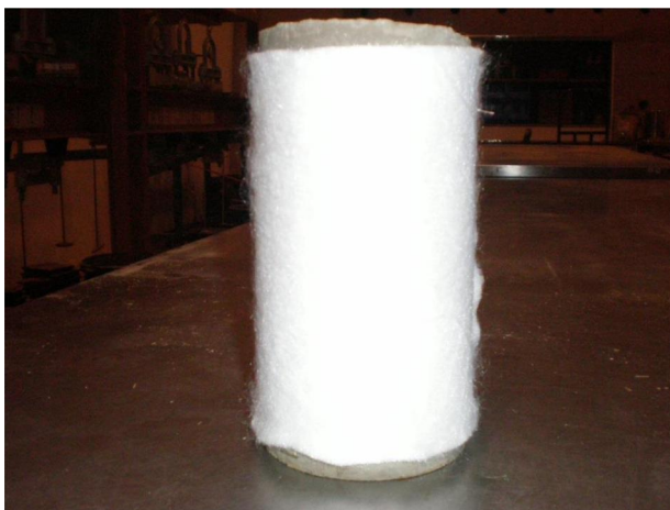
FIG. 6 Hardened RS-CLSM sample reinforced with PET non-woven geotextile.
