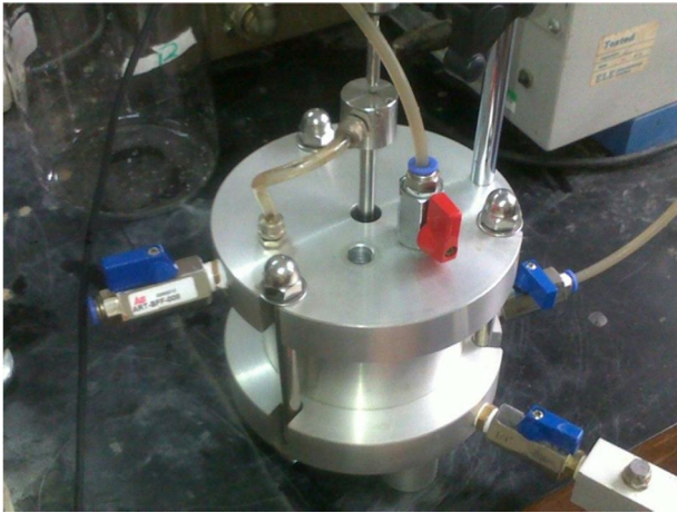
FIG. 1 Rowe cell apparatus.
