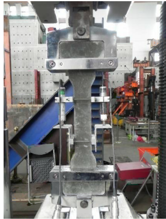
FIG. 3 Direct tensile test setup.
