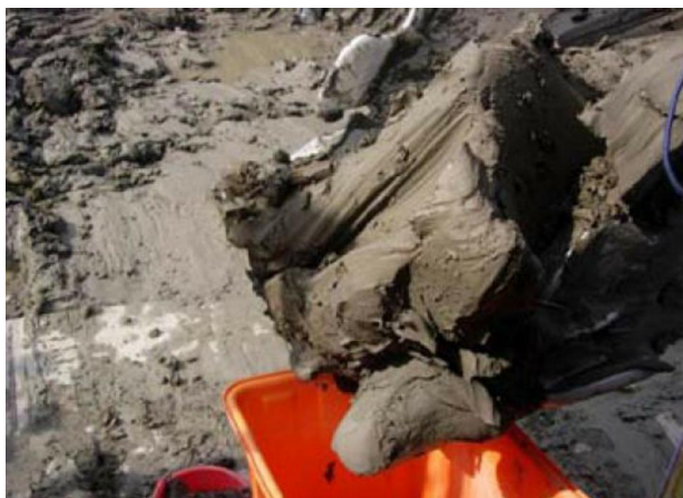
FIG. 3 Sampling of dehydrated dredged reservoir siltation.
