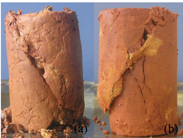
FIG. 13 Images of specimens after shear test: (a) case F; (b) case G.
