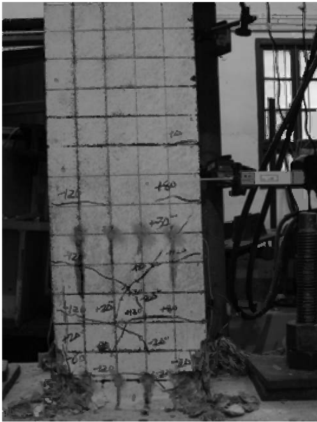
FIG. 9 Failure mode of CE4C.
