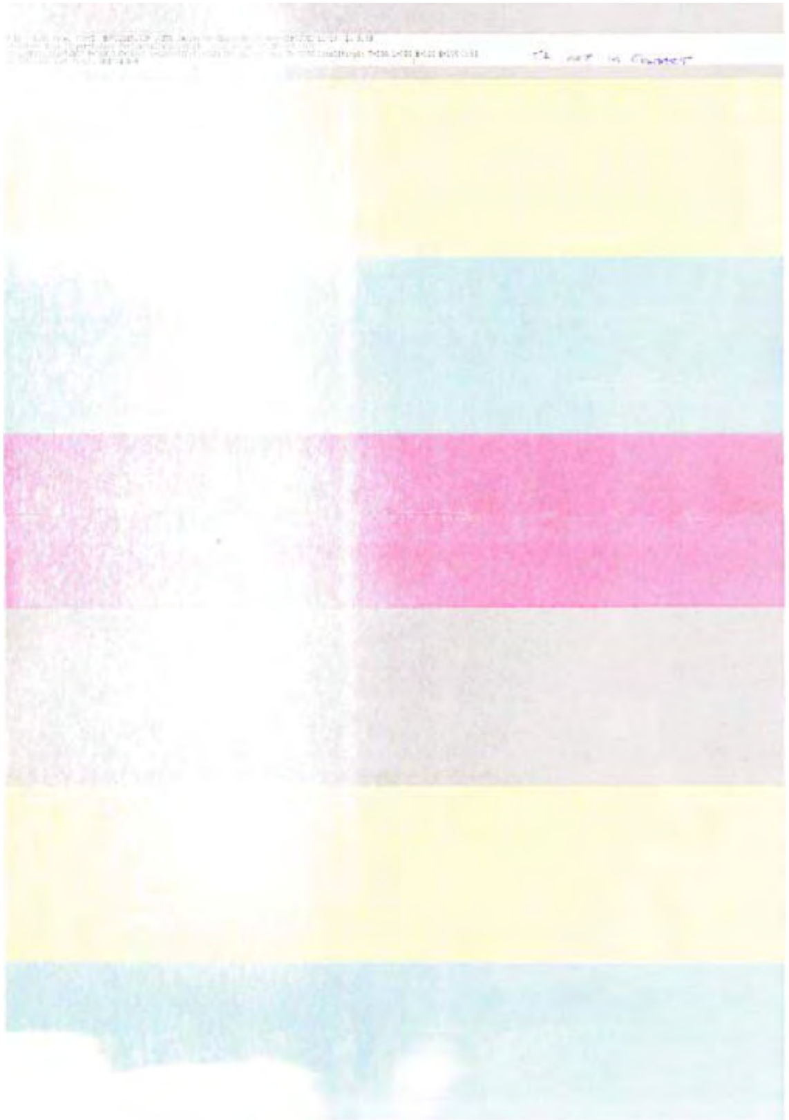
Figure 292. Light or faint image and dropouts
