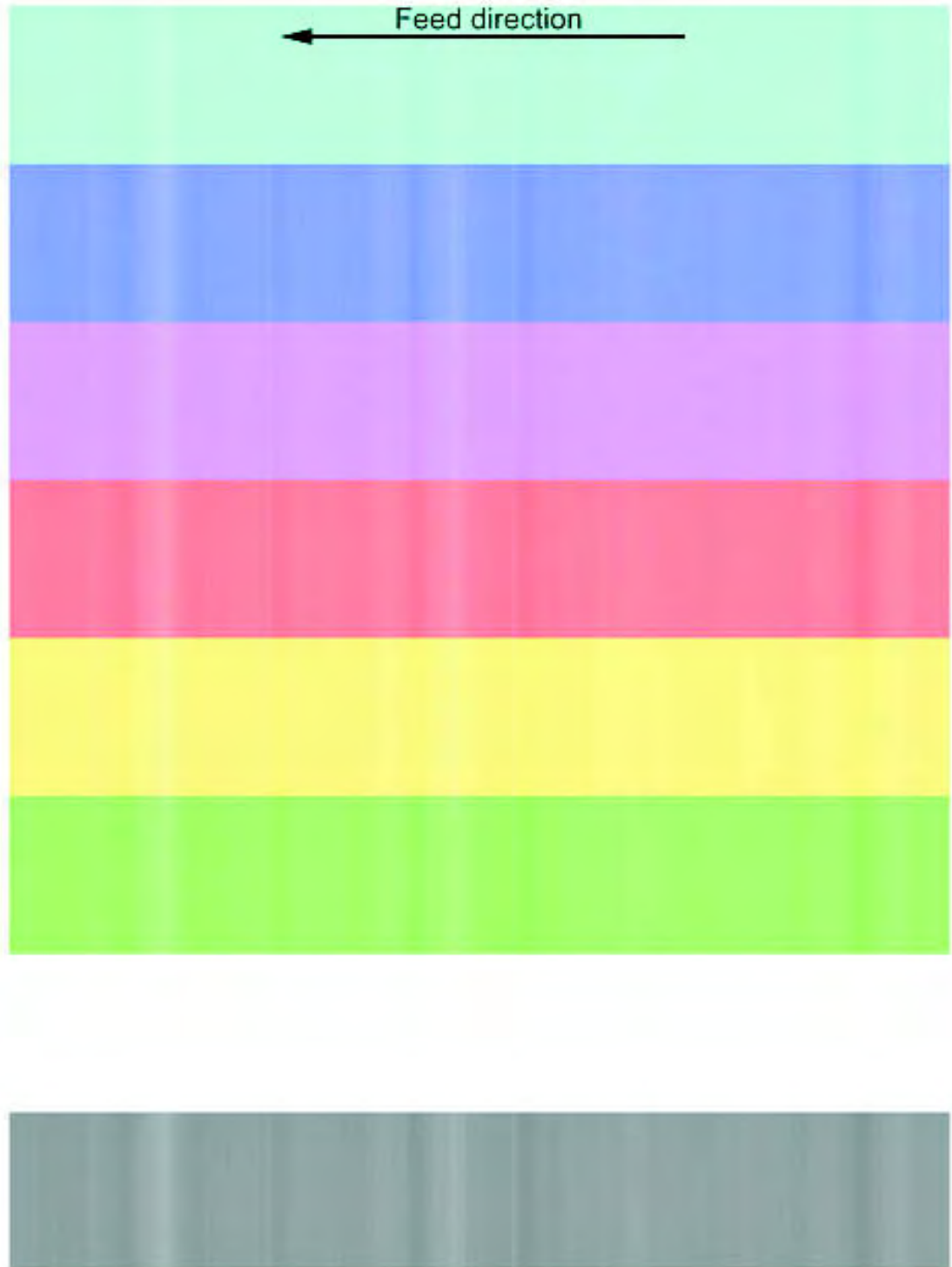
Figure 299. Poorly fused image (1 of 2)
