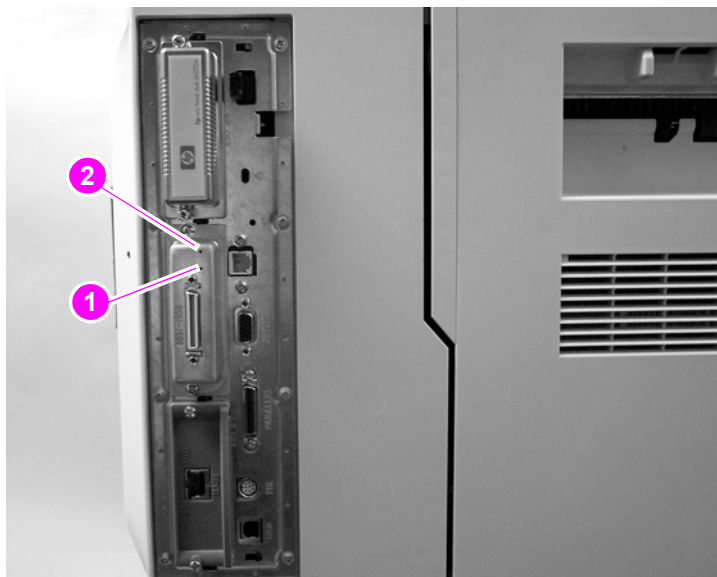
Figure 54. Copy processor LEDs (HP LJ 9040mfp/9050mfp/9500mfp)
