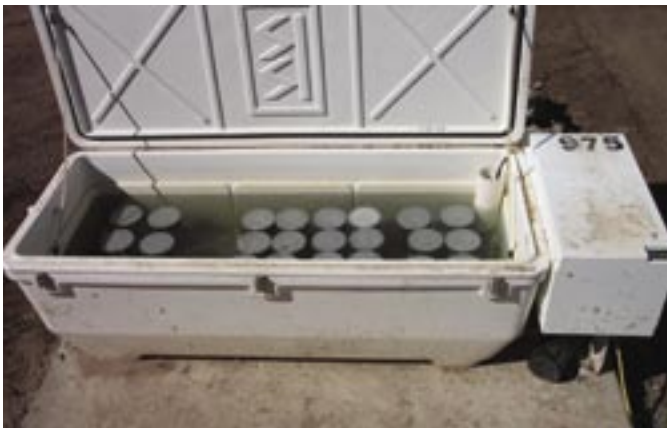
Fig. 1: A thermostatically controlled heating and cooling box can be used to maintain the 60 to 80 °F (16 to 27 °C) initial curing temperature required by ASTM C 31
