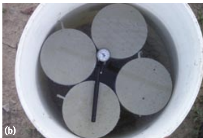
Fig. 3: Pail color affects the water temperature if the pails are left in direct sunlight: (a) water in the black pail was 12 to 15 °F (7 to 9 °C) hotter than water in the white pail; and (b) use a maximum-minimum thermometer to verify that the required 60 to 80 °F (16 to 27 °C) initial curing temperature is maintained
