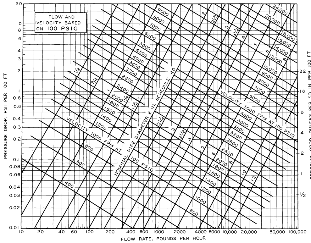
Fig. 13C Flow Rate and Velocity of Steam in Schedule 40 Pipe at Saturation Pressure of 100 psig
