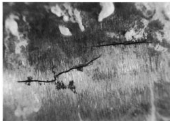
FIG. 2 Typical External Stress Corrosion Cracks (5× Magnification)
