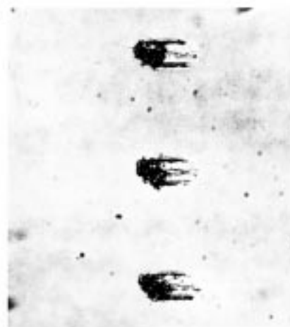
(d) Photograph Showing Three Indentations of a Probe Tip which Moved Laterally on Contact With the Specimen Surface.
