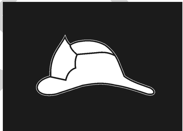
FIGURE 3007.7.5 FIRE SERVICE ACCESS ELEVATOR SYMBOL
