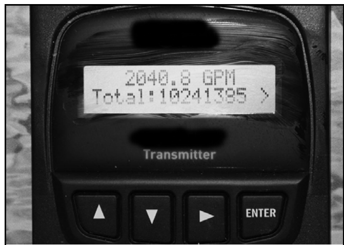
FIGURE 311.7 TYPICAL FLOW METER DISPLAY PANEL
