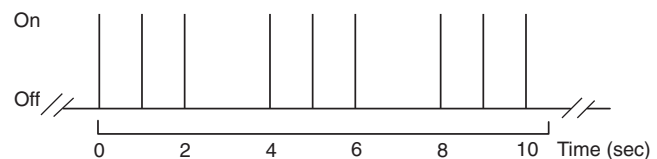
Figure A-3-8.4.1.2(c) Temporal pattern imposed on a single-stroke bell or chime.
