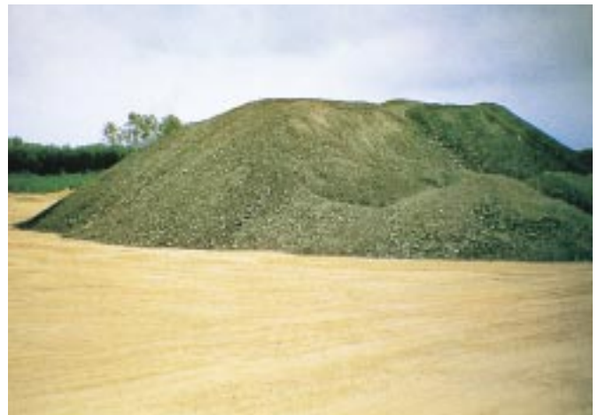
Salvaged Material (RAP) Stockpile
