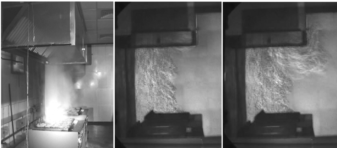
Fig. 3 Hot-Air Plume from Cooking Appliances under Wall-Mounted Canopy Hood A. TEST SETUP: Two charbroilers under 8 ft long wall-mounted canopy hood, cooking hamburgers. B. Schlieren photo of capture and containment at 4400 cfm exhaust rate. Hot, clear air visualization, no cooking. C. Schlieren photo of spillage and containment at 3300 cfm exhaust rate. Hot, clear air visualization, no cooking.
