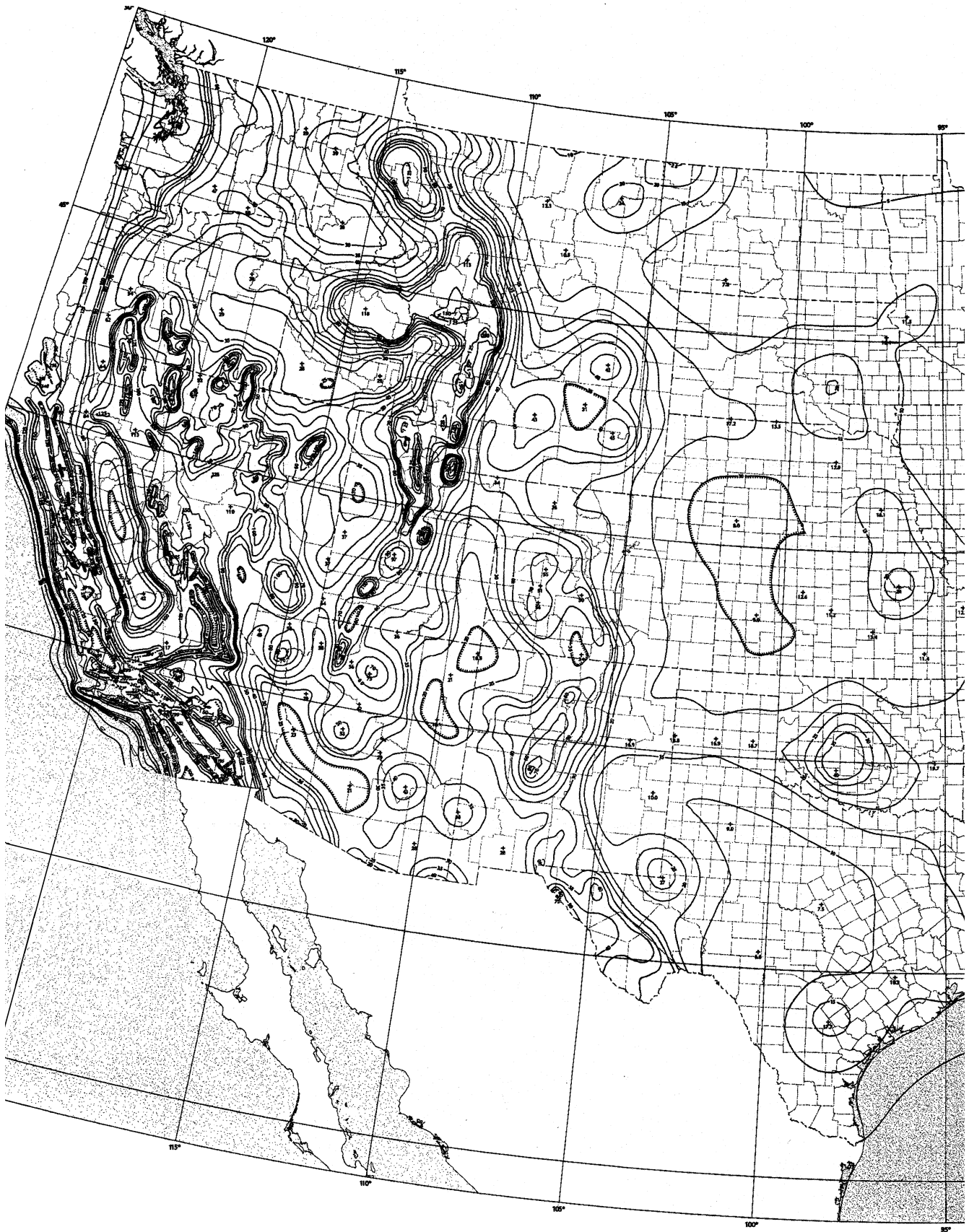
Fig. 1A Maximum Considered Earthquake Ground Motion for the United States 0.2 s spectral response acceleration (% g) (5% of critical damping) Site Class B (Electronic version also available at the USGS web site http://geohazards.cr.usgs.gov/eq )
