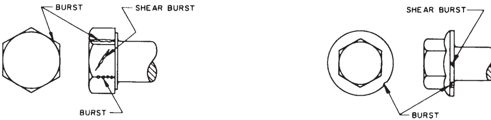
FIG. 3 Typical Bursts and Shear Bursts
