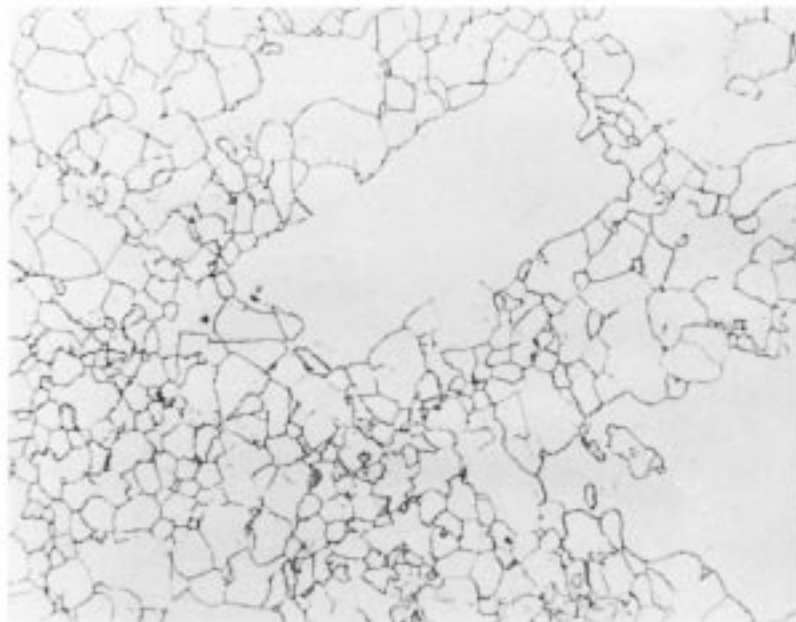
FIG. X2.2 Sample Photomicrograph of Duplex Grain Size 200× Magnification
