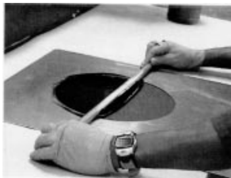
FIG. 3 Emulsion Strike-Off In Template
