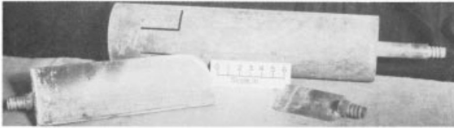
FIG. A1.4 Core Breaker (Lower Right), Core Shovel (Lower Left), and Core Puller (Center)
