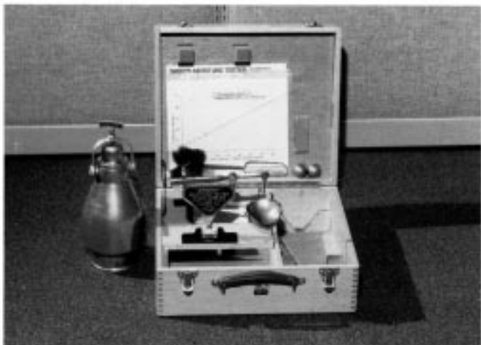
FIG. 1 Typical Calcium Carbide Gas Pressure Test Apparatus for Water Content of Soil
