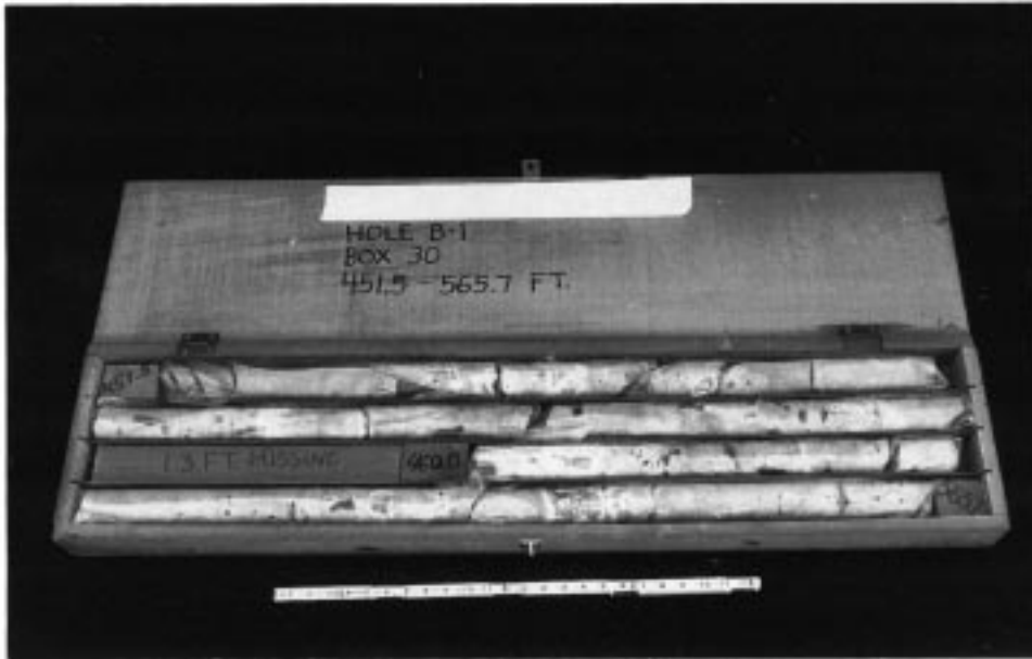
FIG. 2 Typical Wooden Core Box Showing Core Placement, Labeling, and Polyethylene Layflat Tubing Placed Over Core as Suggested for Routine Care (as in 7.5.1)
