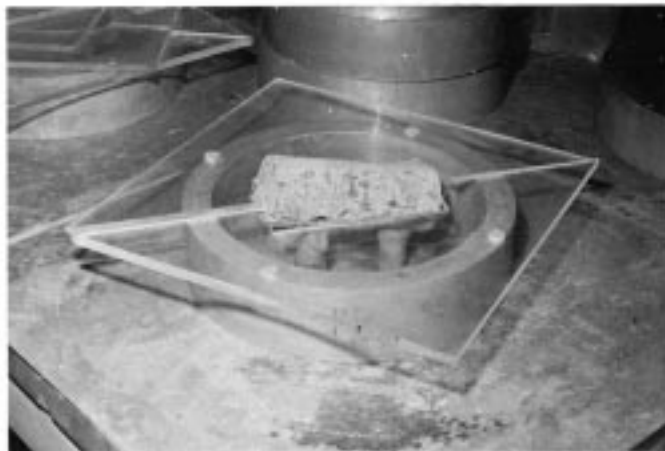
FIG. 5 Specimen Supported in Place By Modeling Clay Pins Which Are Removed After Encapsulating Material Cures and the Resulting Holes Filled With Encapsulating Material
