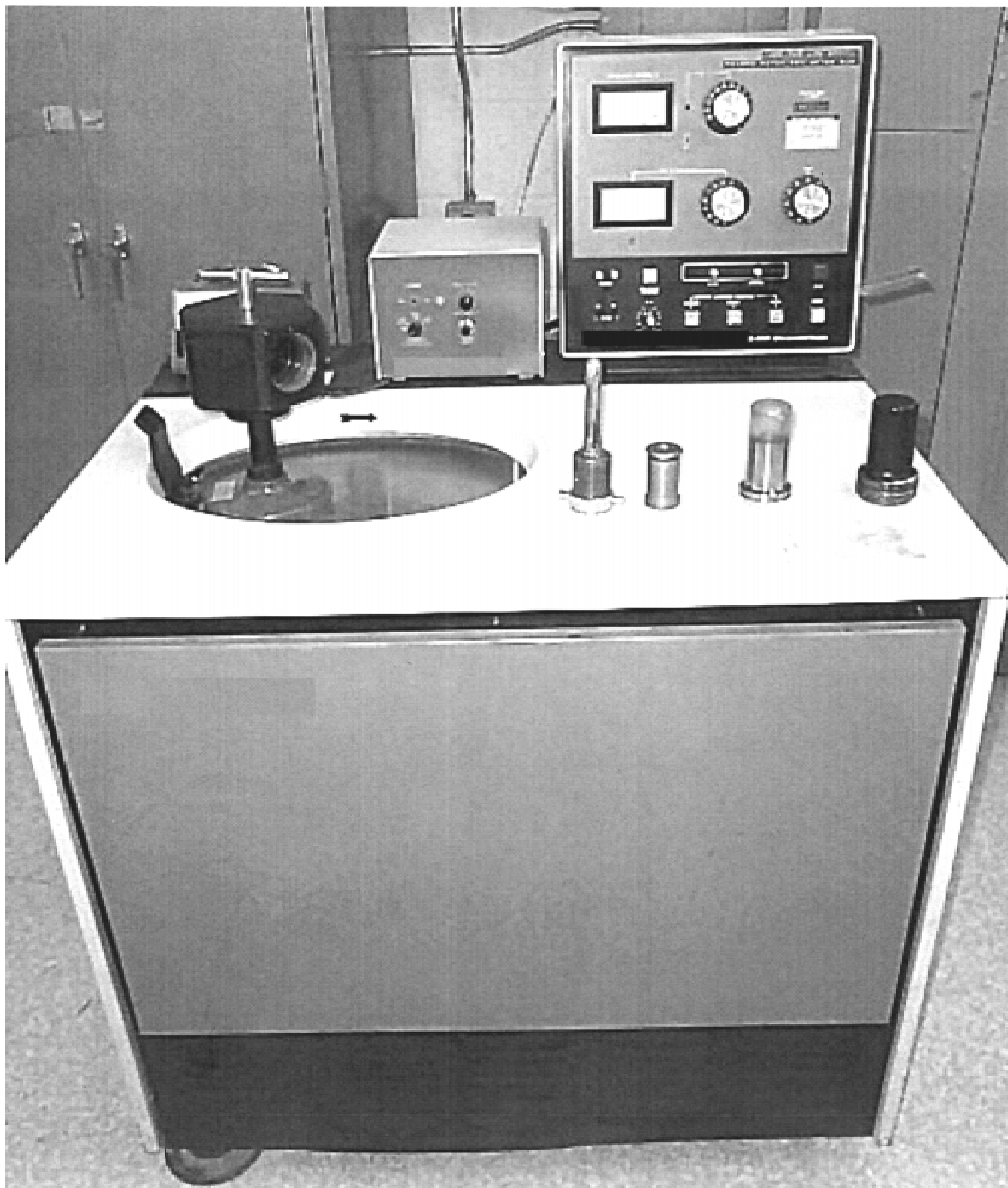
FIG. 8 Photograph of a Temperature-Controlled Centrifuge With Various Specimen Support Chambers
