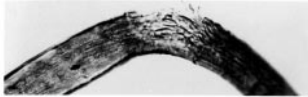
SEMI-RUPTURE AND DEVELOPING SPLIT
