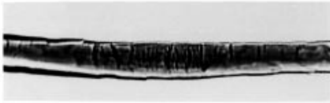
FIBER WITH TRANSVERSE CRACKS
