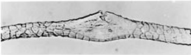
APPARENT SEMI-RUPTURE BUT DO NOT COUNT. CAUSED BY CRACKING
