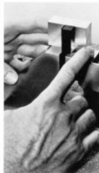
FIG. 4 Jig for Positioning Specimen for Clamping
