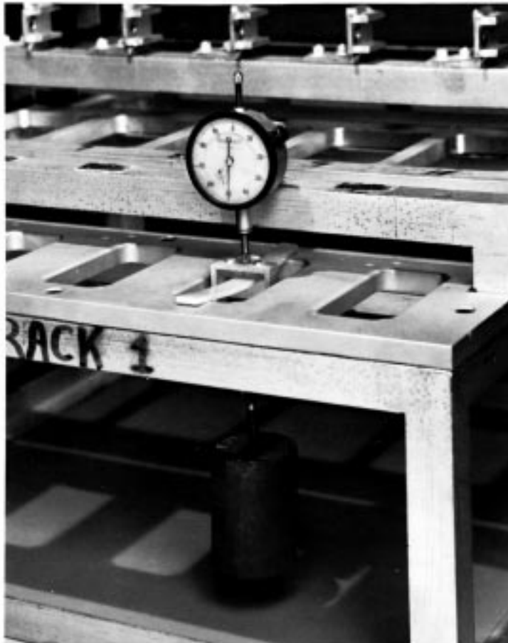
FIG. 2 Flexural Creep Test Apparatus
