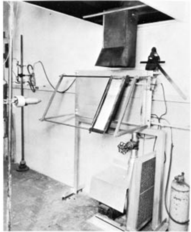
FIG. 1 Radiant Panel Flame Spread Test Equipment
