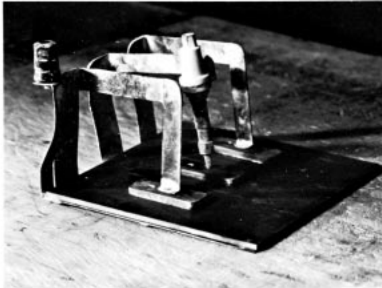
FIG. 4 Clamping Arrangement for Test-Specimen Electrodes
