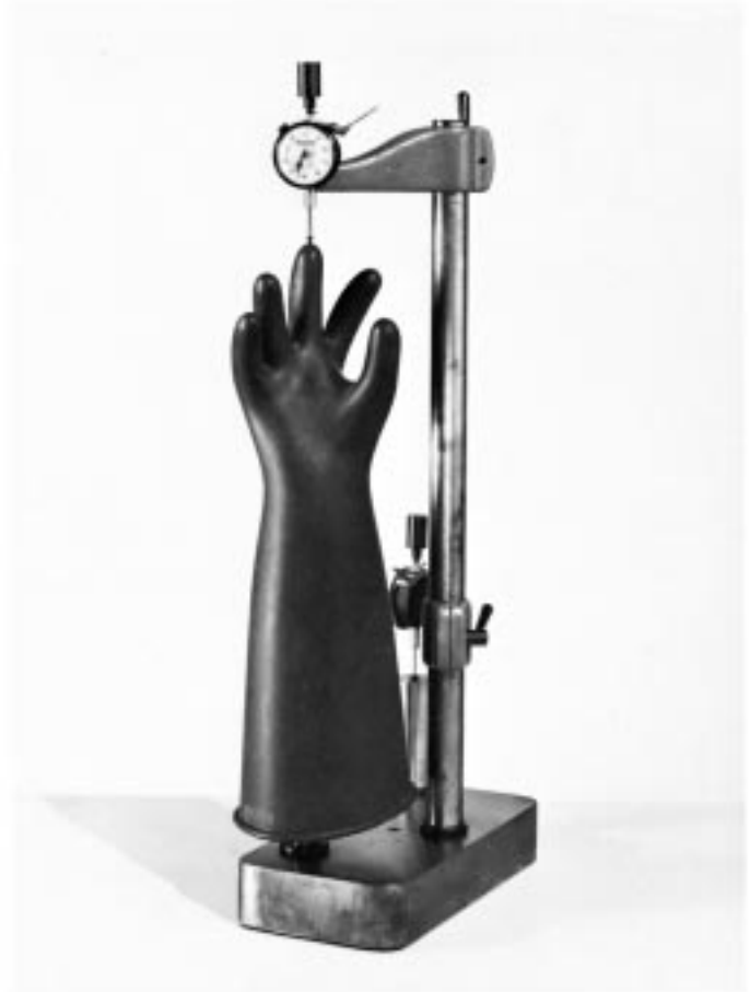
FIG. 4 Dial-Type Micrometer for Measuring Glove Thickness at Fingertips
