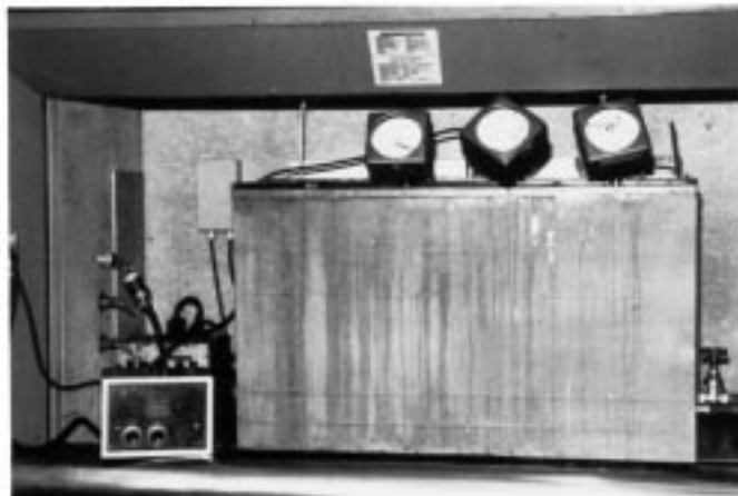
FIG. 1 Rotating Bomb Oxidation Test Apparatus
