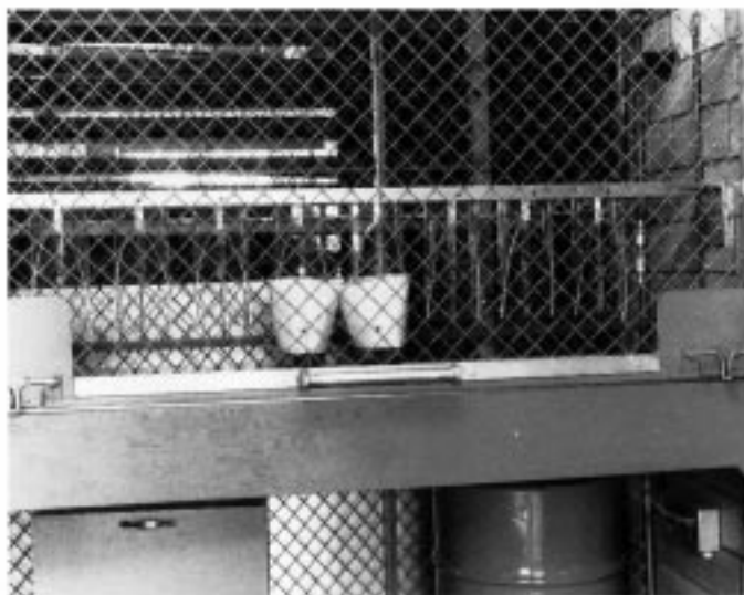
FIG. 2 Typical Test Arrangement for Dielectric Test of Soles of Boots—Enclosure Safety Gate Closed for Test
