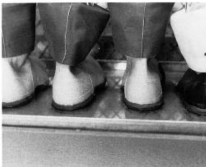
FIG. 4 Typical Test Arrangement for Dielectric Test of Soles of Boots—Boots Standing in Water in Pan Serving as Outer Electrode
