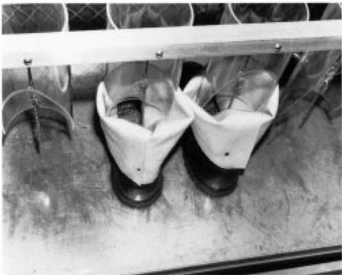
FIG. 1 Typical Test Arrangement for Dielectric Test of Soles of Boots—Shot Electrode Inside Boots, Water Outer Electrode in Pan
