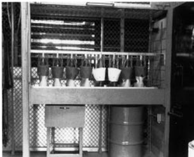
FIG. 3 Typical Test Arrangement for Dielectric Test of Soles of Boots—Enclosure Safety Gate Open
