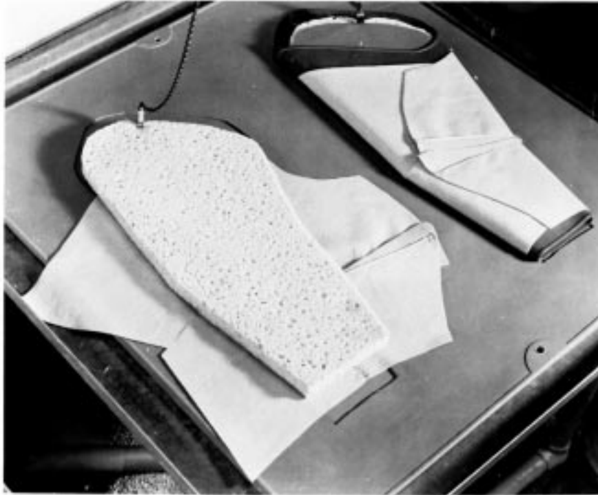
FIG. 7 Wet Sponge Electrode Method
