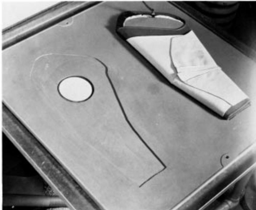
FIG. 6 Wet Sponge Electrode Method
