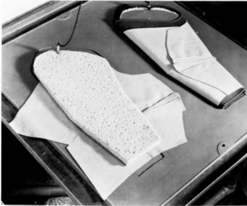
FIG. 7 Wet Sponge Electrode Method
