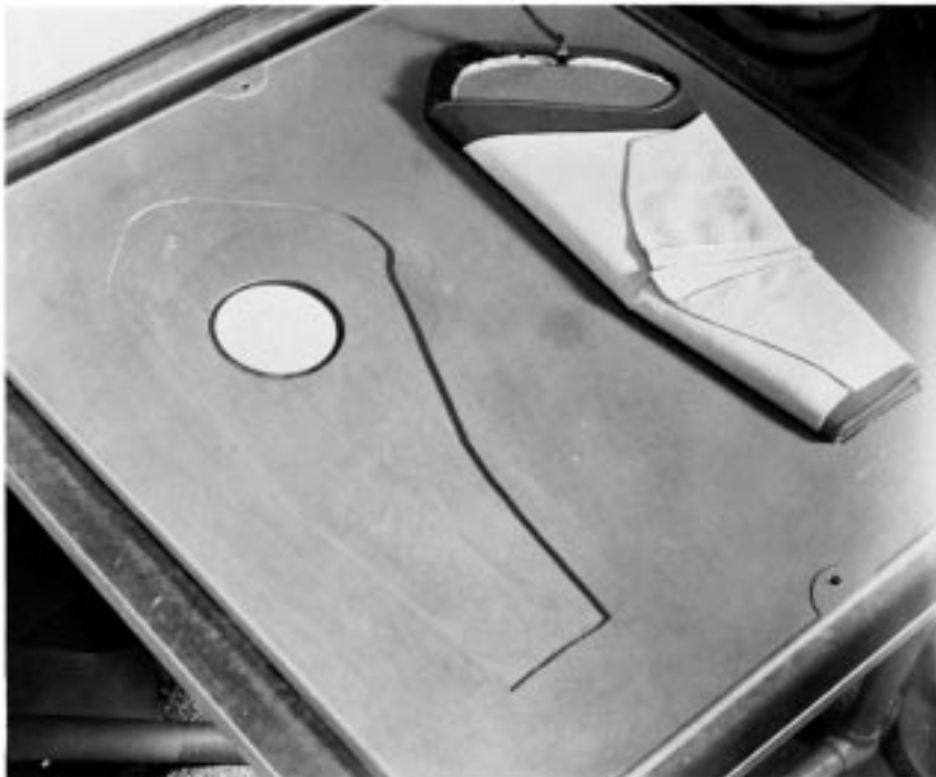
FIG. 6 Wet Sponge Electrode Method
